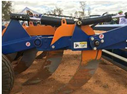
Figure 10b. Grizzly Deep Digger with parabolic tines.
