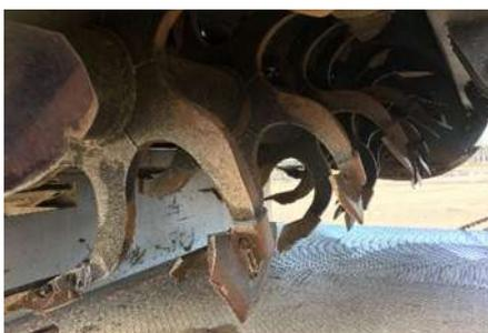
Figure 11a. Triangular shaped spades on curved tines are fixed to a central shaft that rotates at ~90 revs/min<sup>10</sup>.
