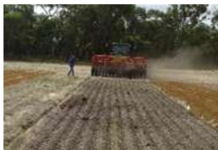
Figure 11b. Press wheels on the back of the spader help to firm the surface and reduce wind erosion risk.
