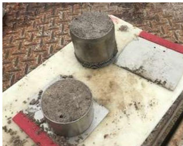
**Figure 7.** Use a steel ring to extract an intact soil core to determine the bulk density.
