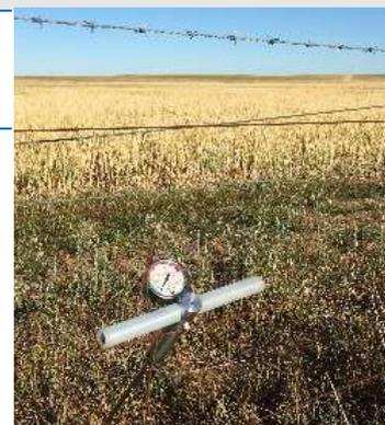
**Figure 6.** An example of an instrumented cone penetrometer, sourced [here](#).
