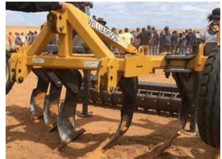
Figure 10c. Williamson-Agri CT ripper with low disturbance Michel tine (curved sideways).
