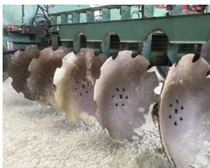
Figure 12a. John Shearer one-way 5GP plough, modified to fit [Plozza](#) discs.
