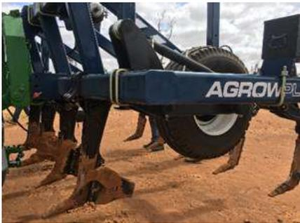
Figure 10a. Example of straight shank tines (AgrowPlover AP51 Ripper) with inclusion plates fitted.
